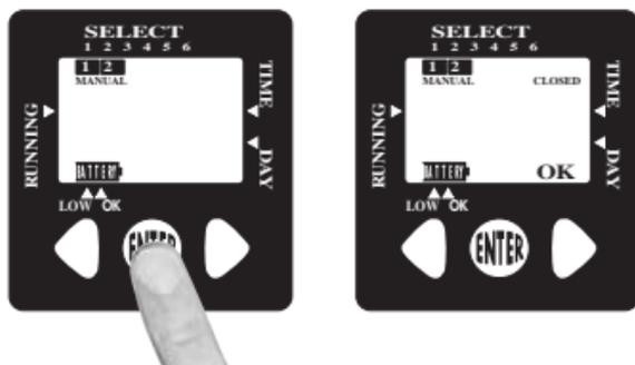
TECLANDO ◀ (OPEN) ABRE-SE A VÁLVULA E TECLANDO ▶ (CLOSED) A VÁLVULA FECHA-SE; DE QUALQUER FORMA, A VÁLVULA FECHA-SE AUTOMATICAMENTE 15 MINUTOS MAIS TARDE.
